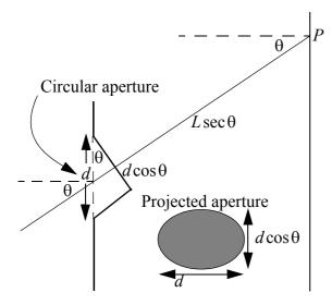
First calculate the solid angle of rays hitting the back of the camera. Viewed from the point P the aperture appears as an ellipse with major and minor axes d and  $d\cos\theta$ . The area of the aperture is therefore
