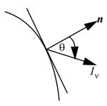
$$F_{v} = \int_{0}^{2\pi} \left\{ \int_{0}^{\pi} I_{v} \cos \theta \sin \theta d\theta \right\} d\phi = \pi I_{v}$$
